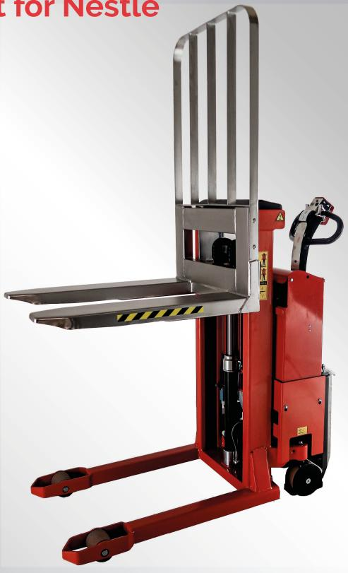
A Logiflex stacker with stainless steel fork chassis and backrest for improved support and safety. The unit operates in Nestlé's production area, where it transports trolleys with trays of biscuits. The stainless parts are to avoid paint contamination of the trolleys.
