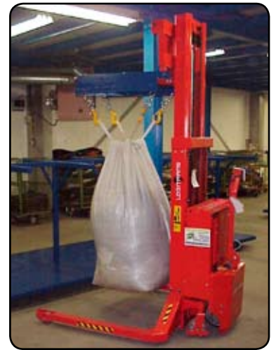
Full Power Straddle Stackers are part of a line that handles second hand clothes. The clothes are checked for damages, and put into big white bags. 03174FC4
