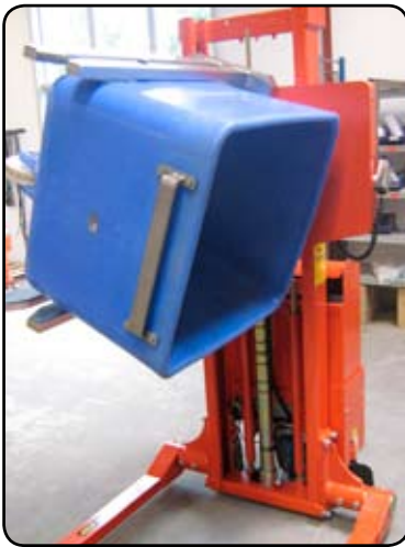
Full Power Stackers with Rotator for the handling of Vemag-containers. Used at a marzipan factory in Denmark. P06692
