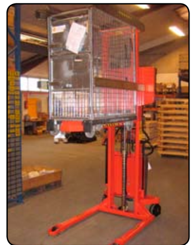
Logiflex ELF with Rotator used at the Swedish postal services for emptying letter containers into sorting machines. P06473
