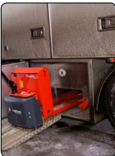
A special low construction makes it possible to place a Panther Maxi AC in a transport box under the lorry during transport. This gives room for two more pallets in the lorry. P04354
