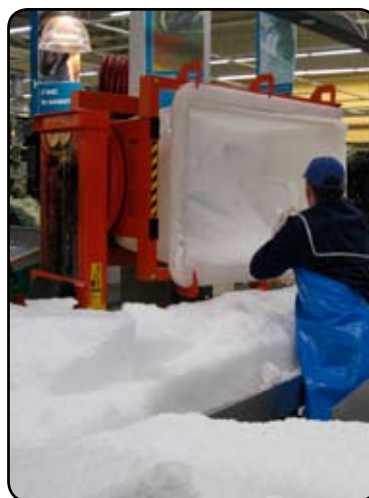
A Full Power Unit with Rotator is used in a supermarket early in the morning to transport ice to the fish department. P05707-2
