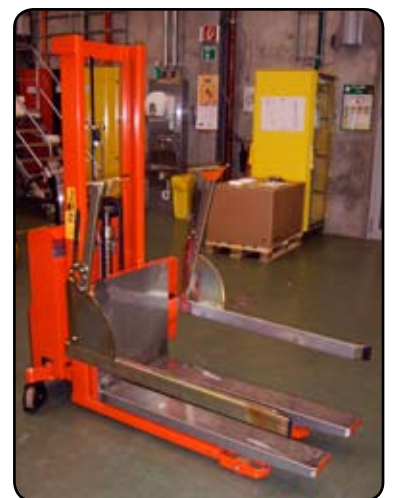
Stacker with Rotator with stainless plating. When transporting stainless containers, they are not damaged and no particles of paint will get in touch with the containers.
