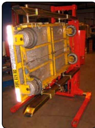
Logiflex straddle stacker with Rotator for the handling of small railway trolleys when carrying through service and repair. P06348-2
