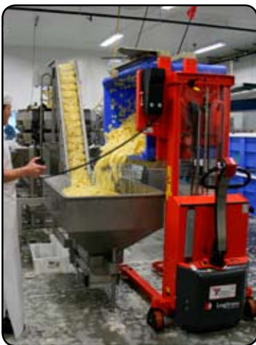
A Norwegian manufacturer of prepared foods for catering centres and groceries uses the fully powered Logiflex with Rotator, when handling vegetables, cream, etc.
