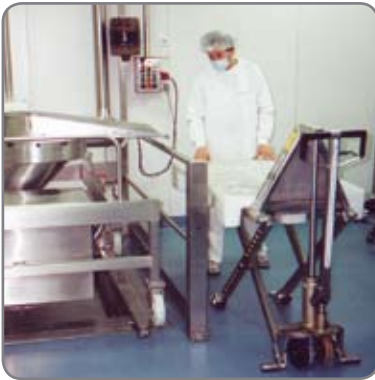
Stainless Thork-Lift ensures an optimum working height.
