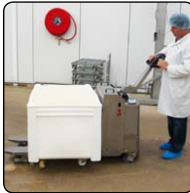
Fully powered pallet truck ensures easy and smooth maneuverability in special environments.
