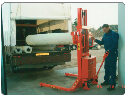
A straddle Trans-Stacker handles reels from a stock to a lorry.
