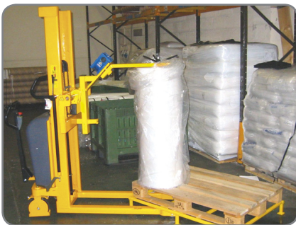
The reel rotator - an ideal alternative when lifting and turning reels.
