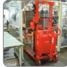
High maneuverability: Short overall length, large turning angle, assisted steering and low own weight.
