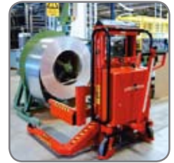
Trans-Positioner with fixed drum fork carriage for the carrying of heavy reels with large diameters.
