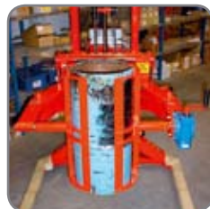
Trans-Stacker with specially made drum turner for drums.
