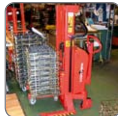
Trans-Stacker with very short forks being used for the handling of wire frames.
