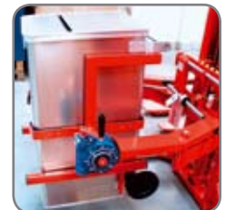
Trans-Stacker revolving a dust-bin (drum turner principle).
