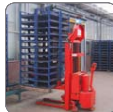
Fully powered Trans-Stacker, remotely controlled from central computer, being used to deliver empty pallets to a production line.
