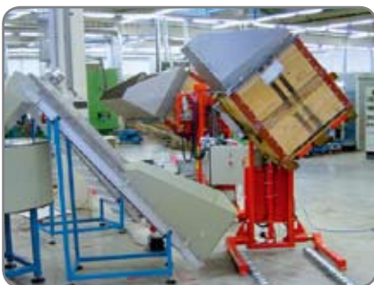
Trans-Stacker with side-tilting forks being used when lifting and emptying components on a production line.
