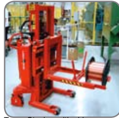
Trans-Stacker with sideways movable carriage with moveable slide. The spool is to be placed on spear at the customer.
