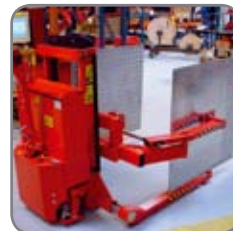
Straddle Trans-Positioner with special gripping arms for light materials.
