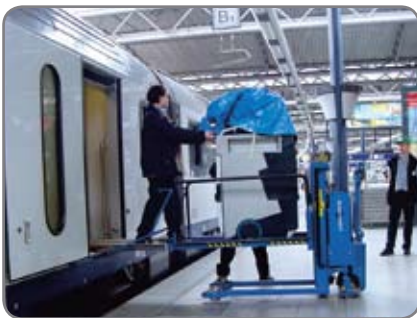
Trans-Positioner with ramp, being used to carry trolleys in and out of trains.
