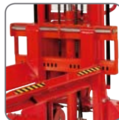
Drum forks are fitted on a special drum fork carriage.
